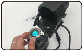
Put the new gobo and fix the jump ring
