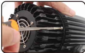
Put the heat sink back and fasten the 4 pcs screws
