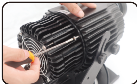
Loosen 4 pcs screws & take apart the heat sink
