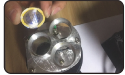
3. take out the old gobo and install the new gobo (Right side face bottom)
